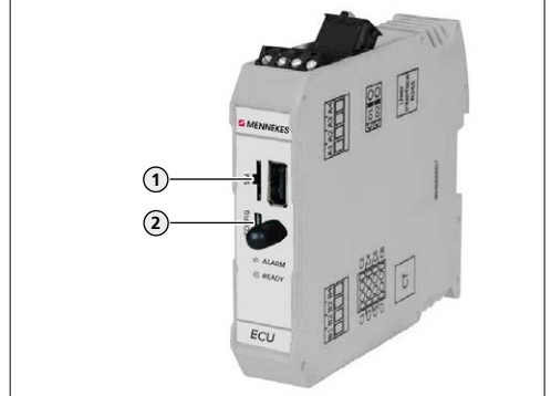
Fig. 14: Connections for the configuration on the ECU
